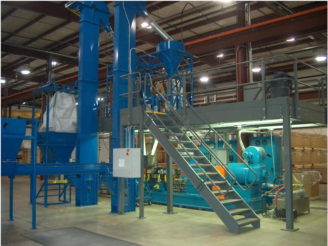
The twin screw extruder is designed and configured to maximize the shearing force on the crumb rubber before it is mixed with the molten plastic in the extruder inducing cross-linking or chemical bonding between the two materials. The compounding temperature is determined by the processing temperature of the plastic (PP, HDPE, LDPE) just as the residence time is determined by the type of
